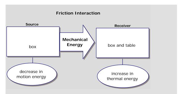
The box slows down because it transfers mechanical energy to the table and the box increasing their thermal energy during this friction interaction.
