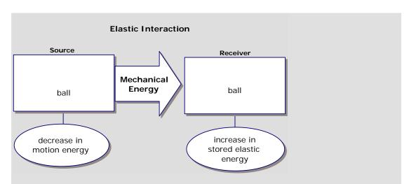
The ball decreases in motion energy as it first interacts with the wall because it transfers mechanical energy to increasing its stored elastic energy. (Note, there is also some sound energy produced when the ball hits the wall)
